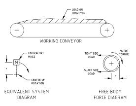
Figure No. 1 Conveyor Inertia
